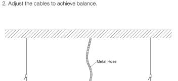
4. Wrap the wires with metal conduit.
