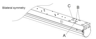
Fix fixture to T-bar ceiling grid with T-bar clips which provided by customer. Refer to the left drawing, fix T-bar clips on Position " C ".
