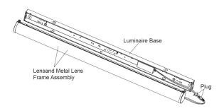
2. Disconnect the wire plug to start installation.
