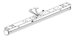
3. Install and lock the mounting plate on the luminaire base following the arrow.
