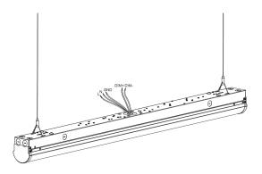
3. Connect the AC wires and dimming wires.
