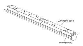
1. Unscrew the 4pcs screws on the back box of the luminaire or the luminaire base.
