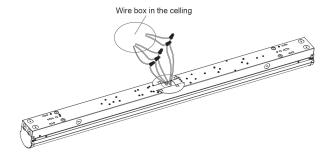
4. Connect the AC wires and dimming wires.
