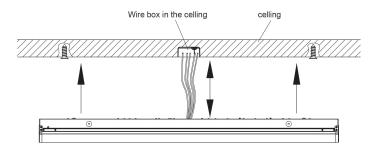
5. After wire connection complete, fix the screws on the ceiling.
