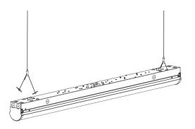
1. Clip the aircraft cable into the planned holes.
