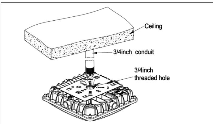
1. Make the wiring connection, and insert the wires inside the conduit. Rotate the fixture clockwise until it is secured.
