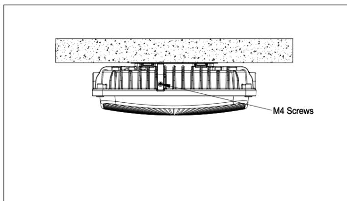
3. Hook the fixture into the spindle on the mounting plate, and make sure fixture is properly secured. Make the wiring connection, and insert the wires inside the junction box, and push the fixture toward the ceiling.
