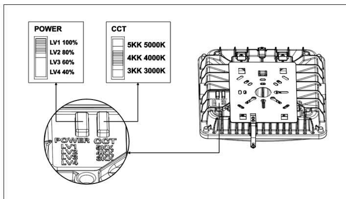
1. Power and CCT can be adjusted by sliding into the desired level as shown.
