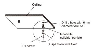
1. Install the suspension wire fixer on the ceilnig, and make adjustment as necessary
