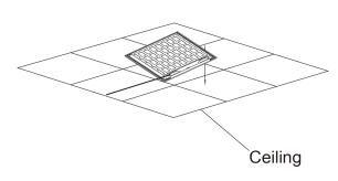
5. Pull the panel down towards the surface of the ceiling, and make adjustment as necessary to have it flush against the ceiling.
