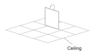
4. Rotate the panel light 90° in vertical direction to make it correspond to the recessed frame and be sure the front of the panel is facing the ground.
