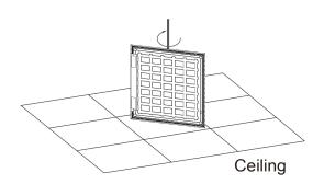
3. Rotate the panel light 45° in horizontal direction to make the front of panel face the ceiling square hole.
